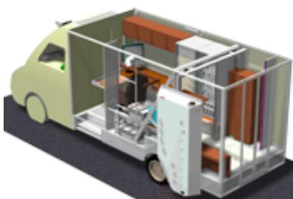
The **Greenwood Profiler** is delivered with a high performance computer with Ethernet network and modular subsystems, which can be plugged-in and synchronized. A multifunctional solution is operated from a keyboard connected to a rack mounted PC, which controls the data acquisition and subsystems.
