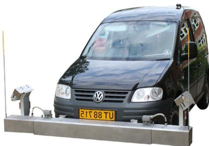
**Greenwood Profiler** can be operated as a standalone system or part of a multifunction vehicle.
