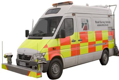
**Greenwood Profiler** gives both transverse and longitudinal profile, and allows them to be combined in one 3D profile.
