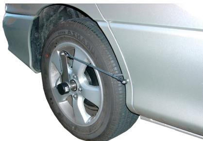
An odometer is mounted on the wheel of the vehicle and in combination with the inertial system. It keeps precise track of the vehicle movement. Each laser provides a longitudinal roughness profile (IRI) and contributes with one point to the transverse profile. The lasers can be upgraded to texture lasers (64 kHz) that also measures the texture profile (MPD).
